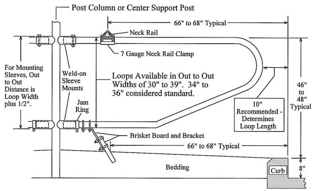
Loop lengths are manufactured based upon bed depths, and widths to customer desire. Actual lengths may vary 1/2" +/-. Distance from bottom of loop to bedding is determined by loop width selection and height of mount.
